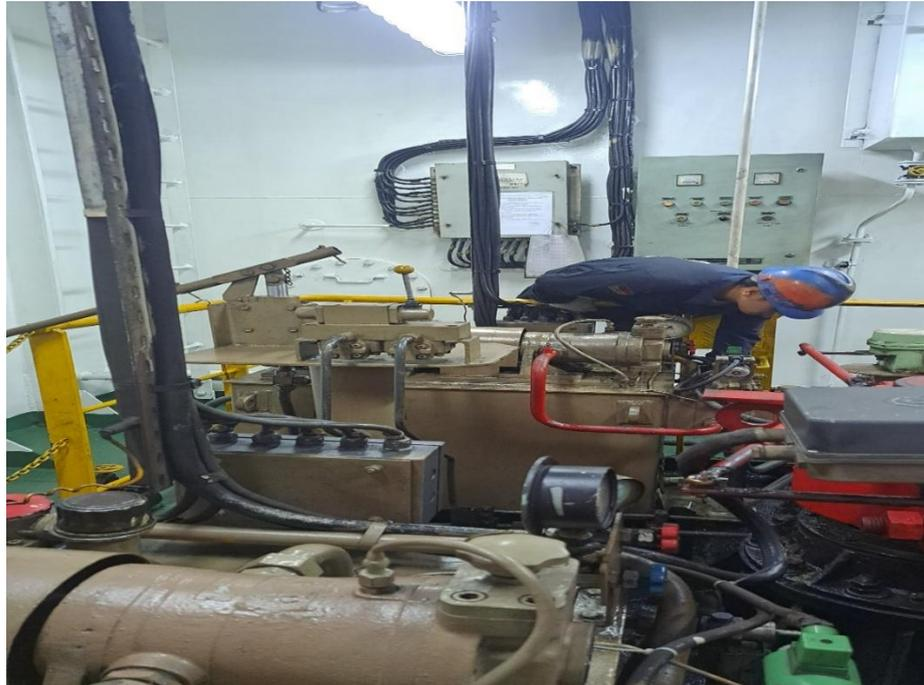
***Pengecekan Oil Level Steering Gear***
