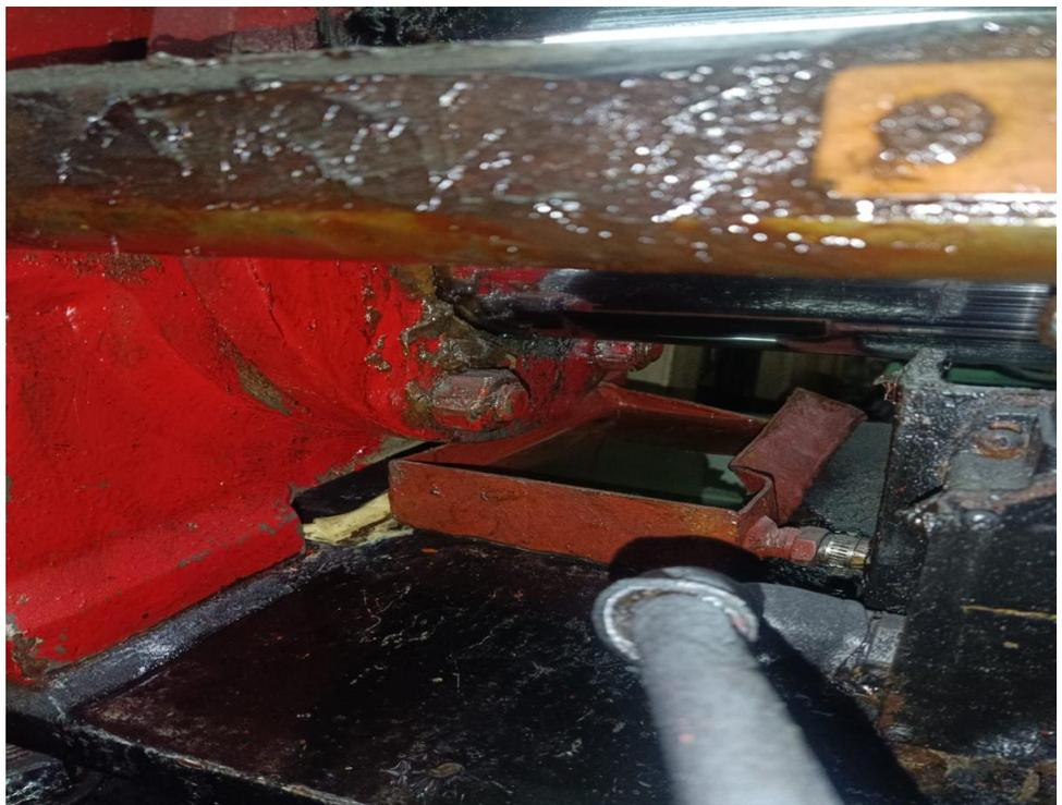
***Kebocoran Pada Shaft Steering Gear***
