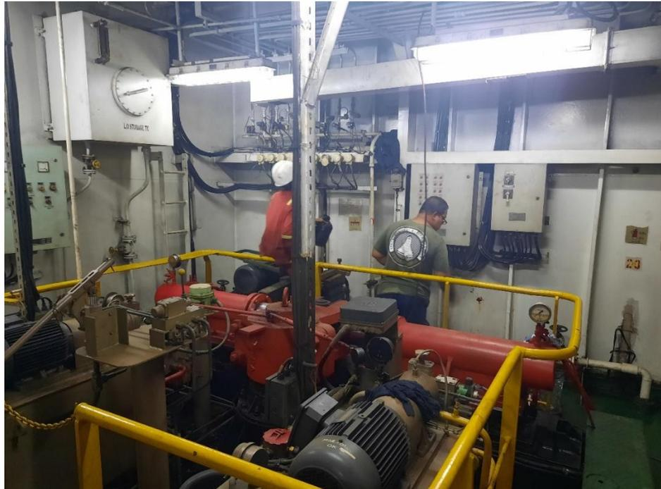
*Pengecekan Sistem Steering Gear Oleh Teknisi*
