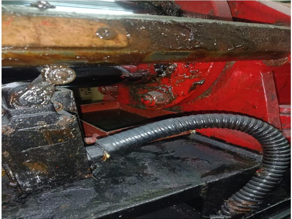
***Kebocoran Pada Shaft Steering Gear***
