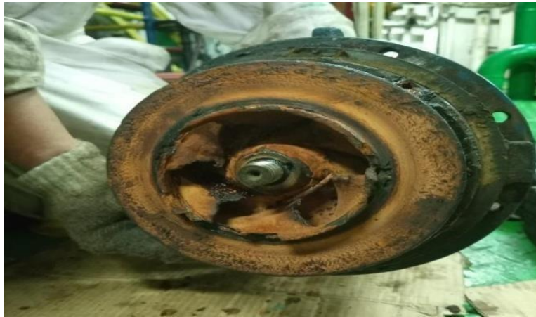
Gambar 3.4 Overhaul pompa pendingin MT. Sea Reliance
