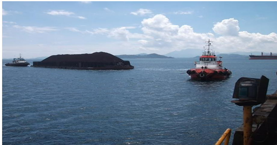
Gambar 4.8 Proses Tugboat Menarik Tongkang Berisi Muatan
