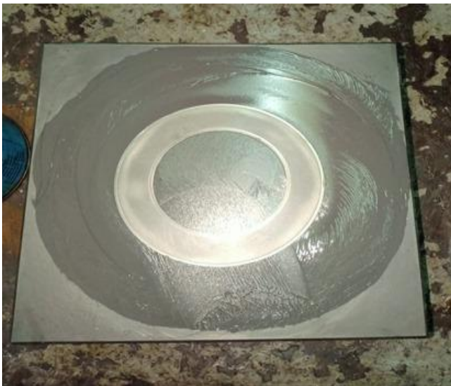
GAMBAR:LAPPING DISK DAN VALVE HIGHT PRESURE ,LOW PRESURE KOMPRESSOR UDARA
