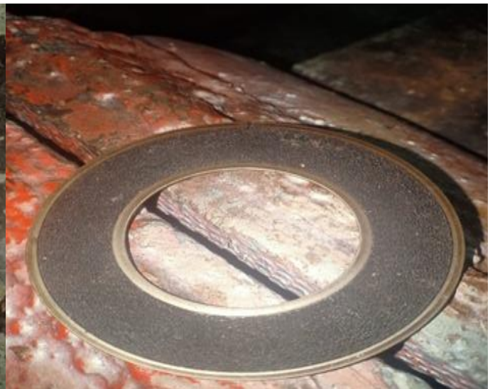
GAMBAR:LAPPING DISK DAN VALVE HIGHT PRESURE ,LOW PRESURE KOMPRESSOR UDARA
