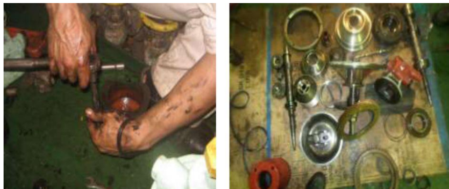
Gambar 4.6 proses overhaul LO Purifier
