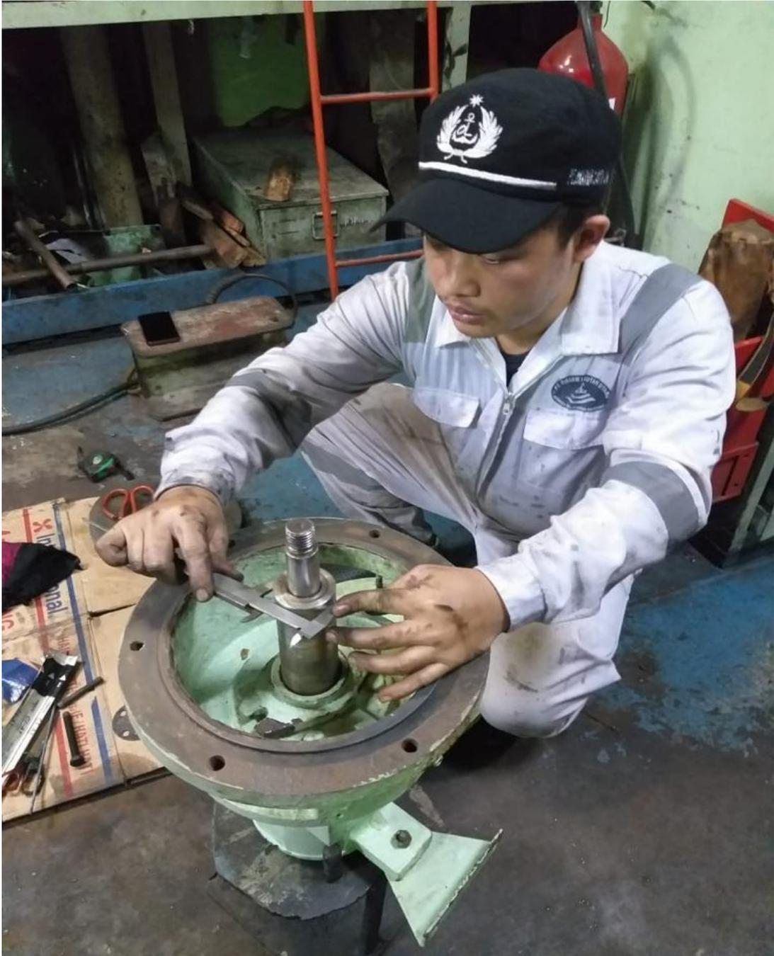
Gambar : Mengukur Poros Fresh Water Pump
