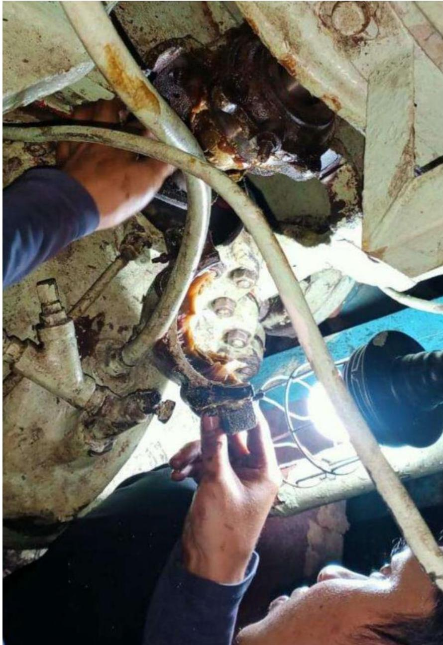
Gambar : Penggantian Packing Fresh Water Pump
