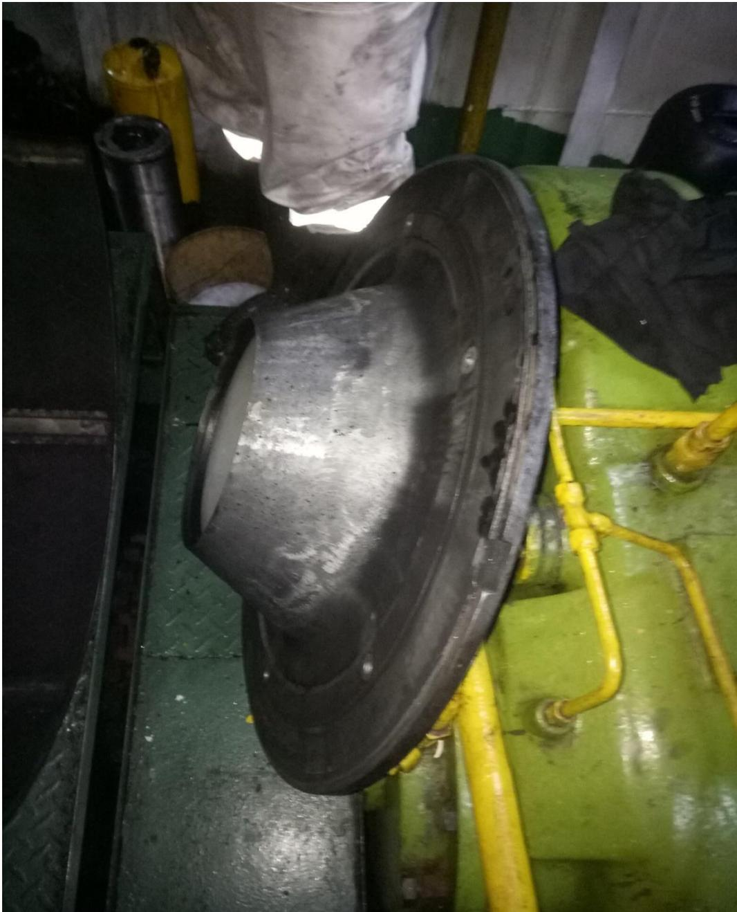
Gambar: Cover depan Turbocharger MV . SELARAS MAS
