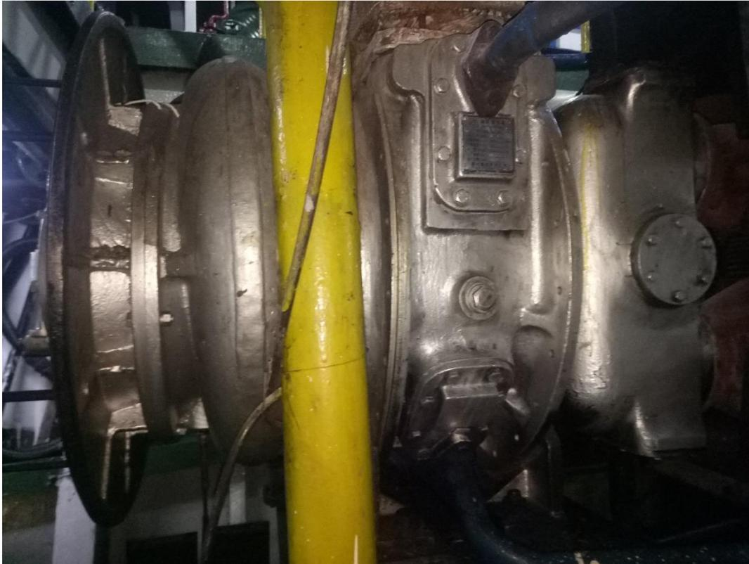
Gambar: Body Turbocharger MV . SELARAS MAS
