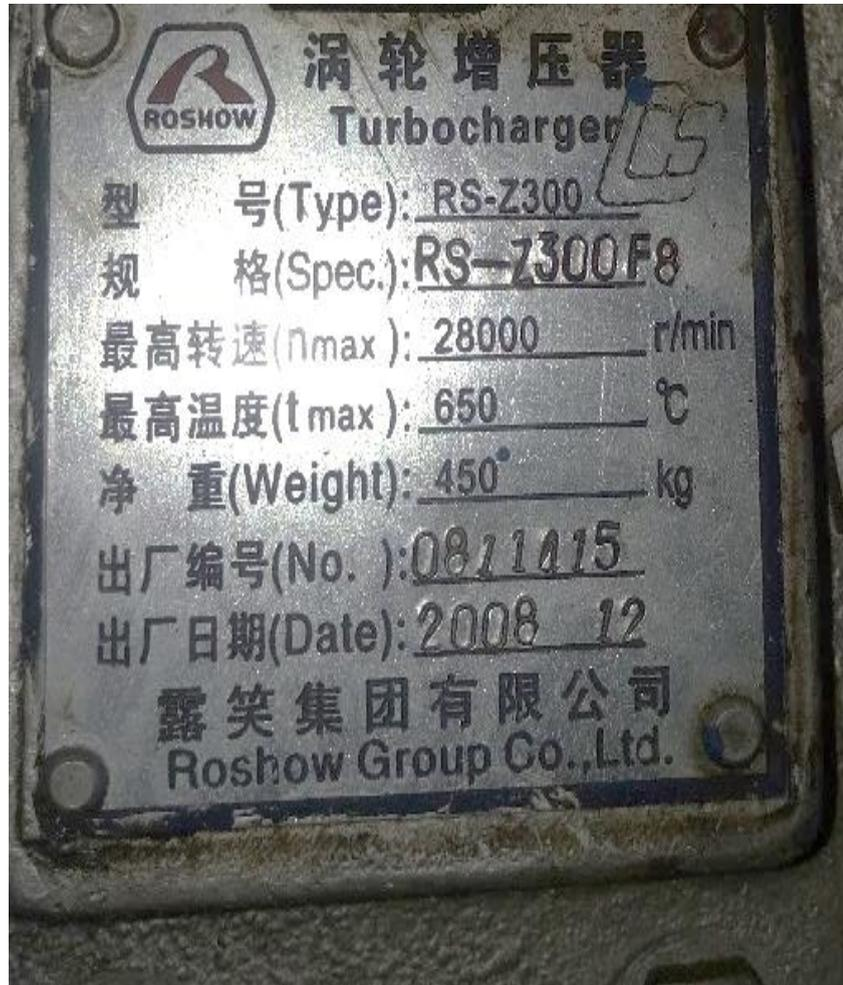
Gambar: Name Tag Turbocharger MV . SELARAS MAS
