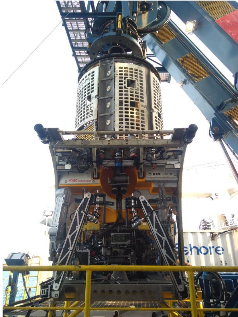
Gambar 3. ROV (Remotely Operated Vehicle) milik kapal Surf Allamanda
