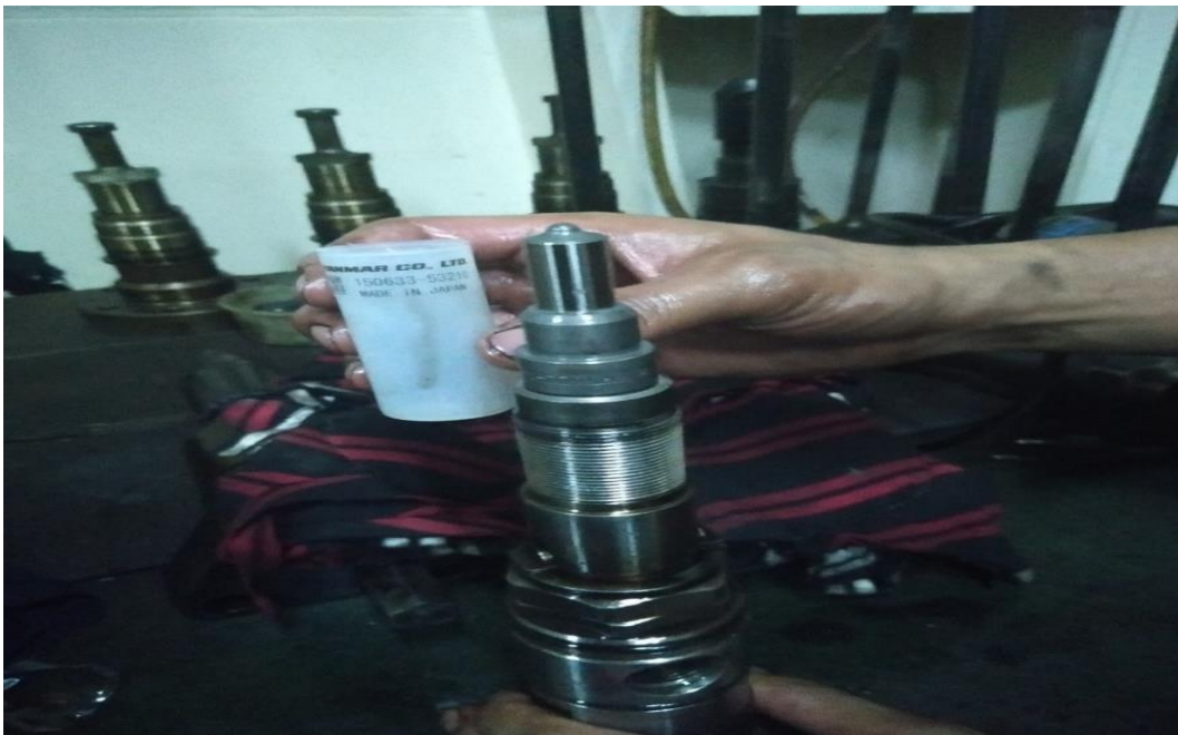
Gambar : Pergantian Nozzle Baru Sumber : MV. Dian Prosperity
