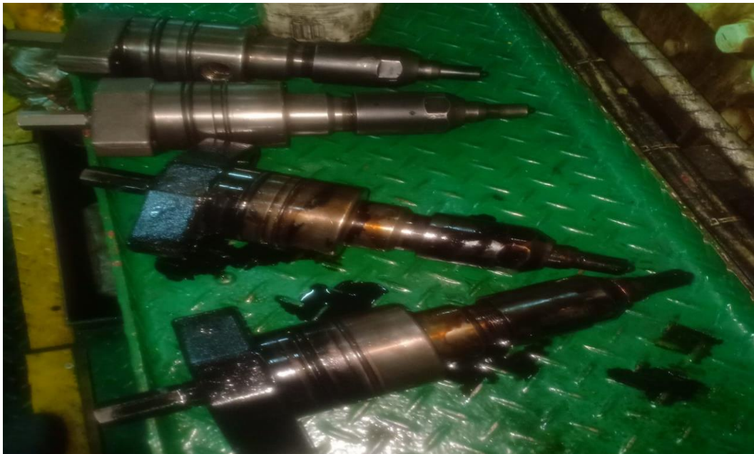
Gambar : Injector Menetes Sumber : MV. Dian Prosperity
