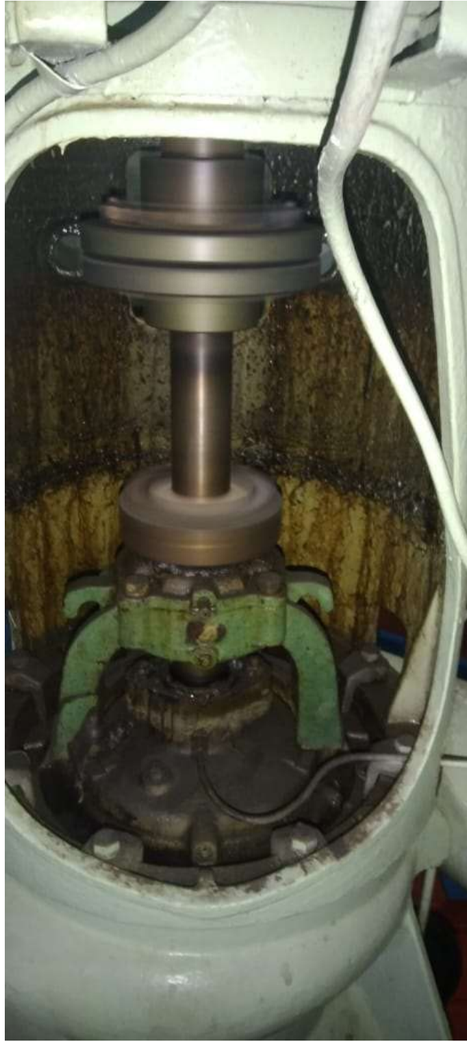
Gambar : Poros (as) Fresh Water Pump Sumber : KM. Dharma Kartika IX, 2021
