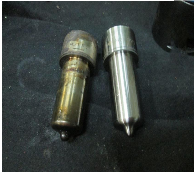
Lampiran 10: New nozzle and old nozzle
