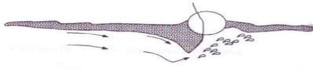
Gambar 4. 7 Oil Boom Failure-Drainage
