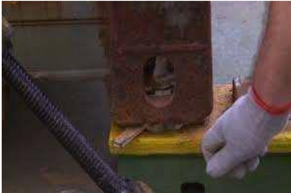
Gambar 2.4 Manual Left Locking Twistlock
