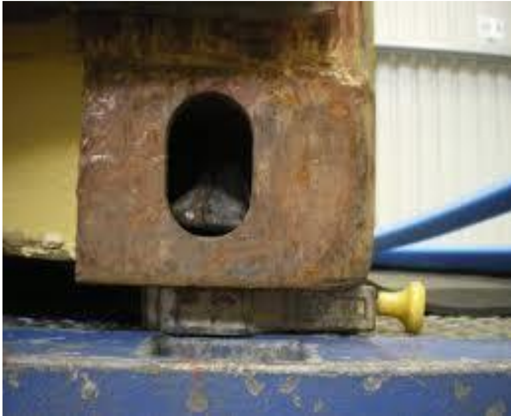
Gambar2.3Semi Automatic Twist lock
