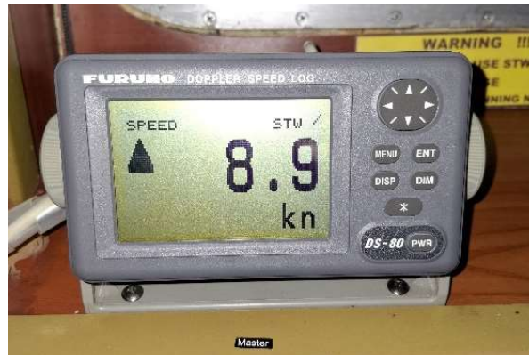
Gambar 2.6 Doppler Speed Log
