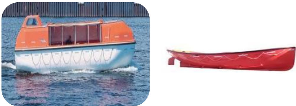
Gambar 2.2 Semi Enclosed Lifeboat dan open Lifeboat
