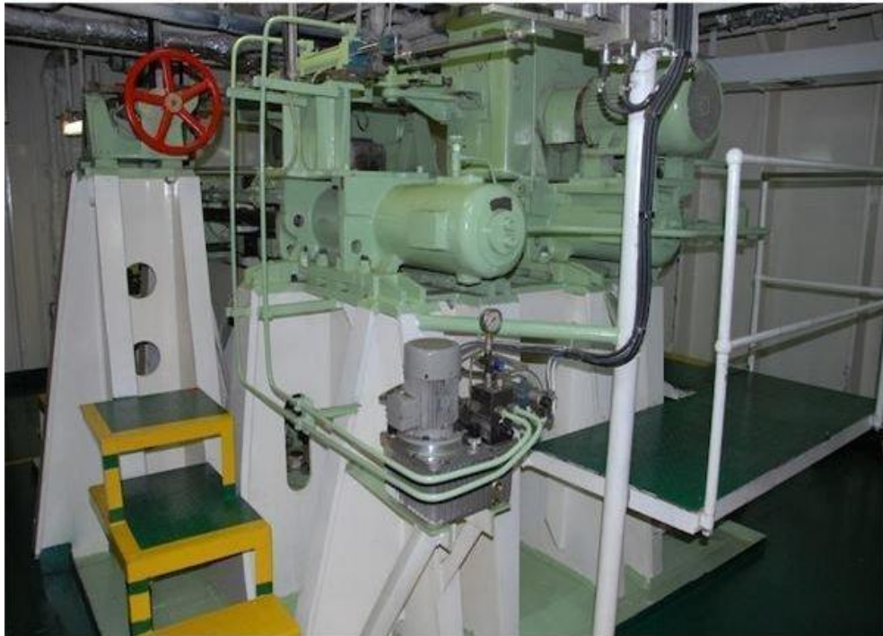
Gambar 2. 4 Hydraulic Steering Gear
