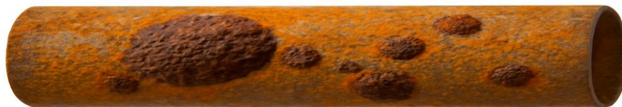
Gambar 2. 6 pipa korosi mikrobiologis
