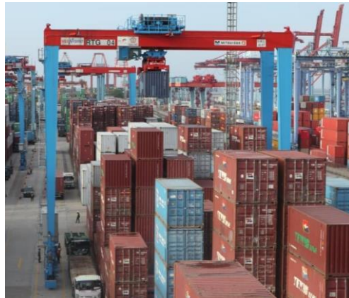
Gambar 2. 3. Rubber Tyred Gantry (RTG) Crane
