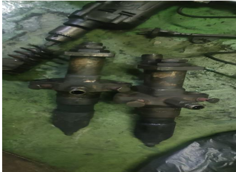
Gambar 2.3 Injektor/ Fuel Injection Valve
