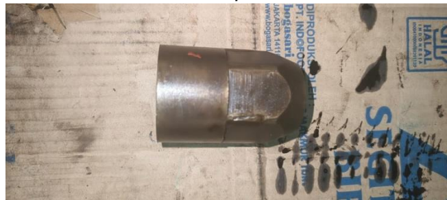
Gambar 2.11 Cap Nut For Nozzle
