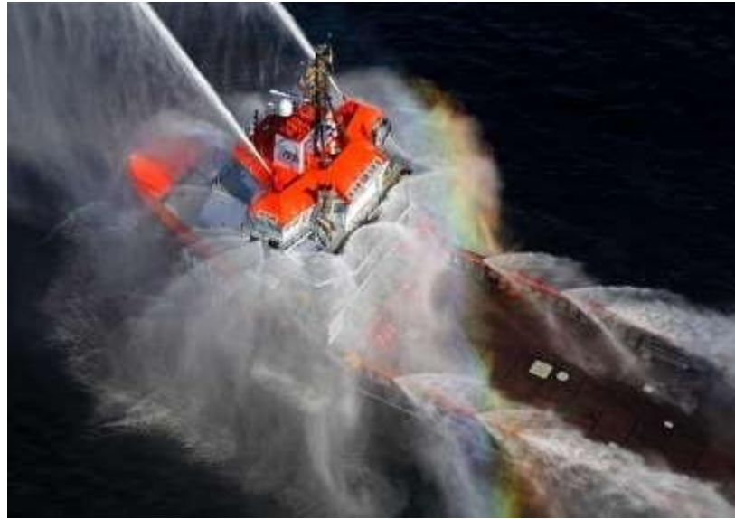
Gambar 5 Water Spray Systems
