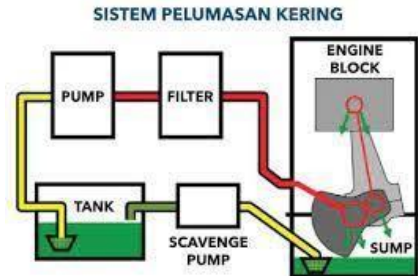
Gambar 2. 8 Dry Lubricating System
