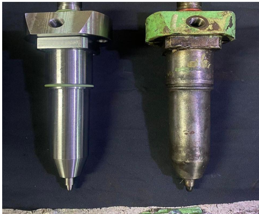
Gambar 2.7 Injector nozzle berlubang satu (single hole)
