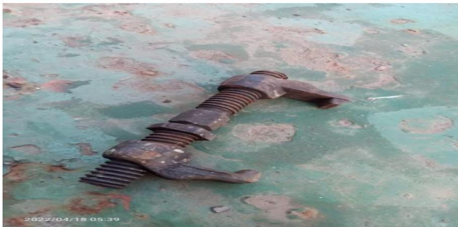
Gambar: 2.17 *screw bridge fitting*
