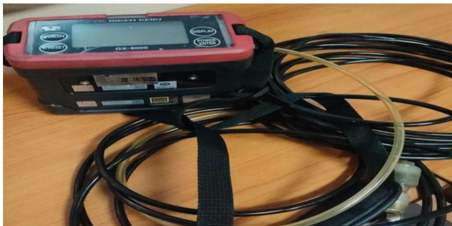
Gambar 2.7 Portable Gass Detector
