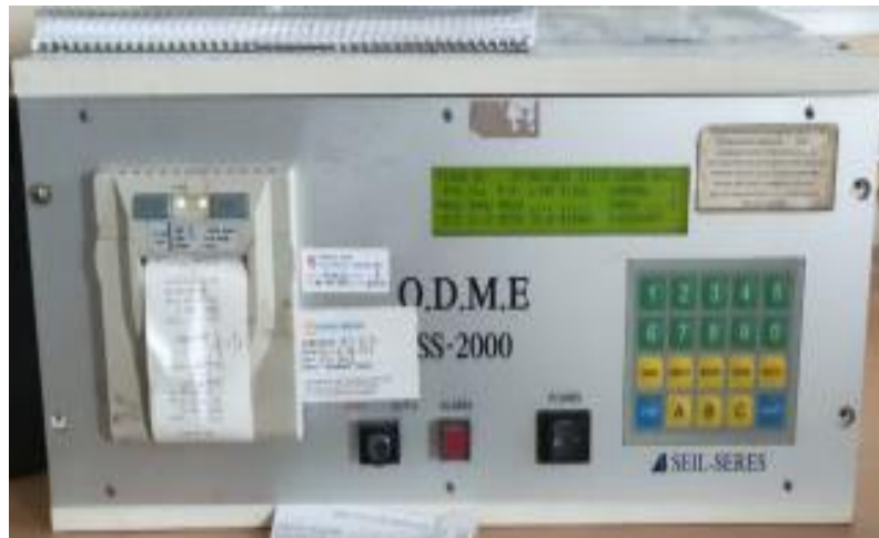
Gambar 2 9. Oil Discharge Monitoring
